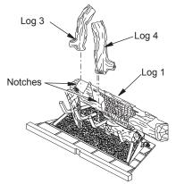
Figure 30 - Installing Logs 3 and 4
